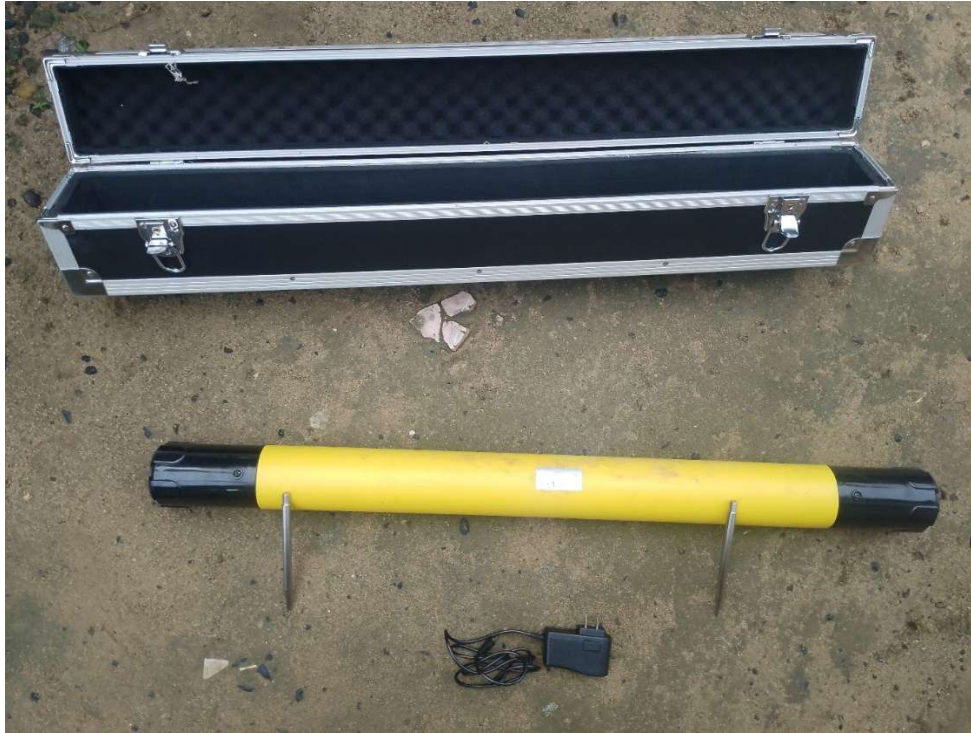
Figure 2: A digital Terrameter for Groundwater Exploration.
