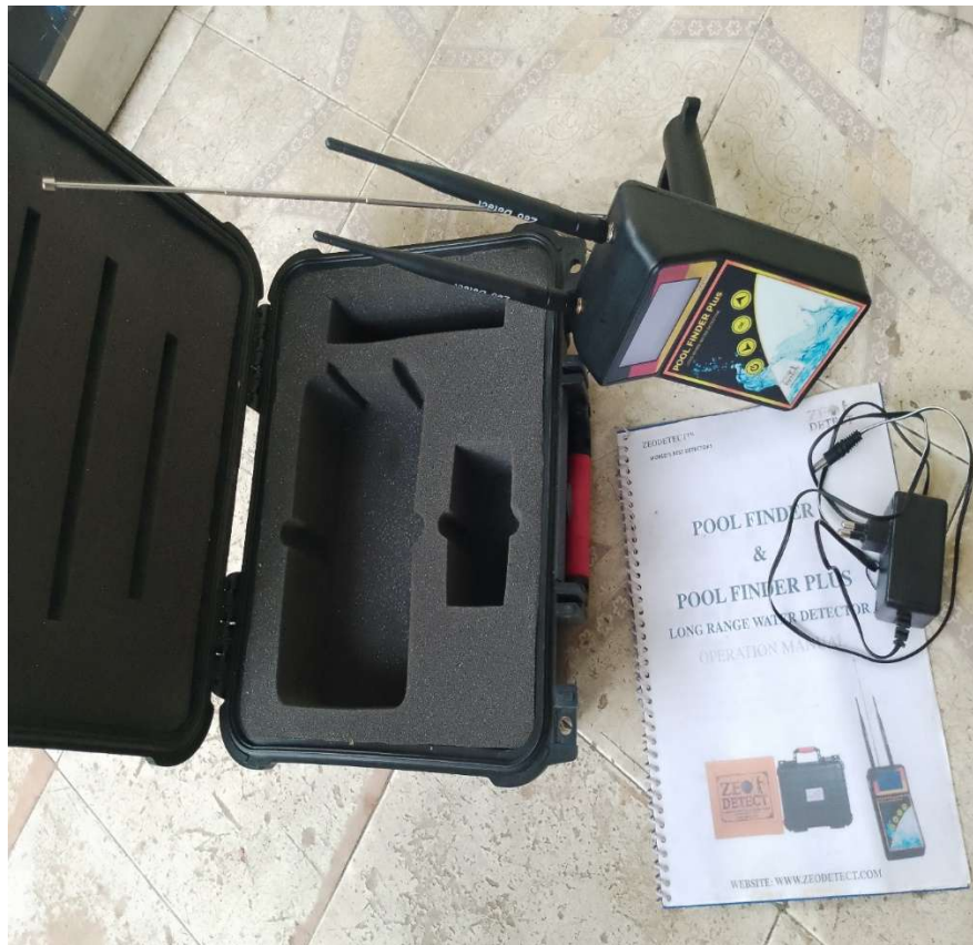
Figure 3: A Pool Finder Plus for Groundwater Exploration.
