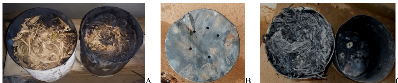
Fig.3: Different stages of carbonization: (A) First carbonization (failure), (B) Bucket drilled to improve ventilation, (C) Second carbonization (successful).
