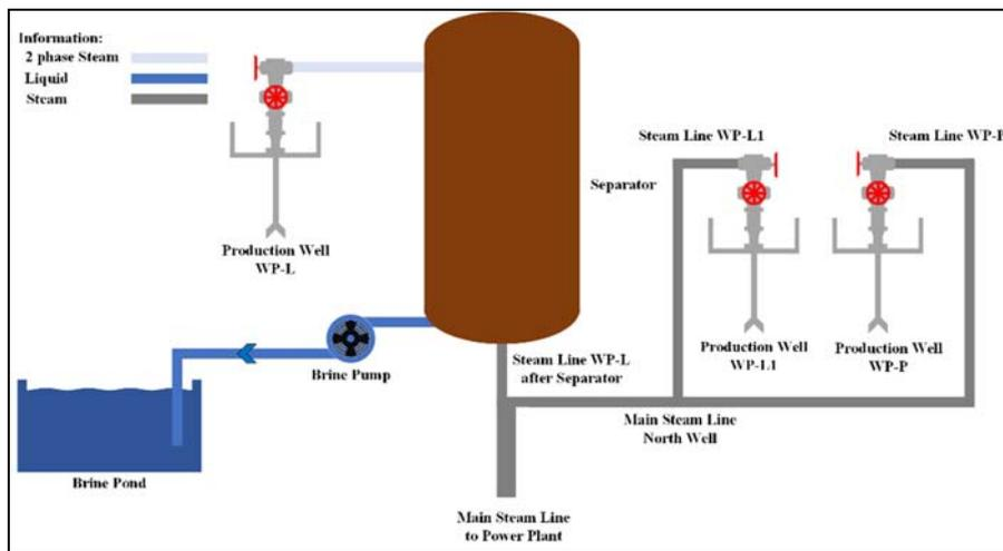
Fig. 1. Distribution Steam WP-L in Separated Steam Cycle
