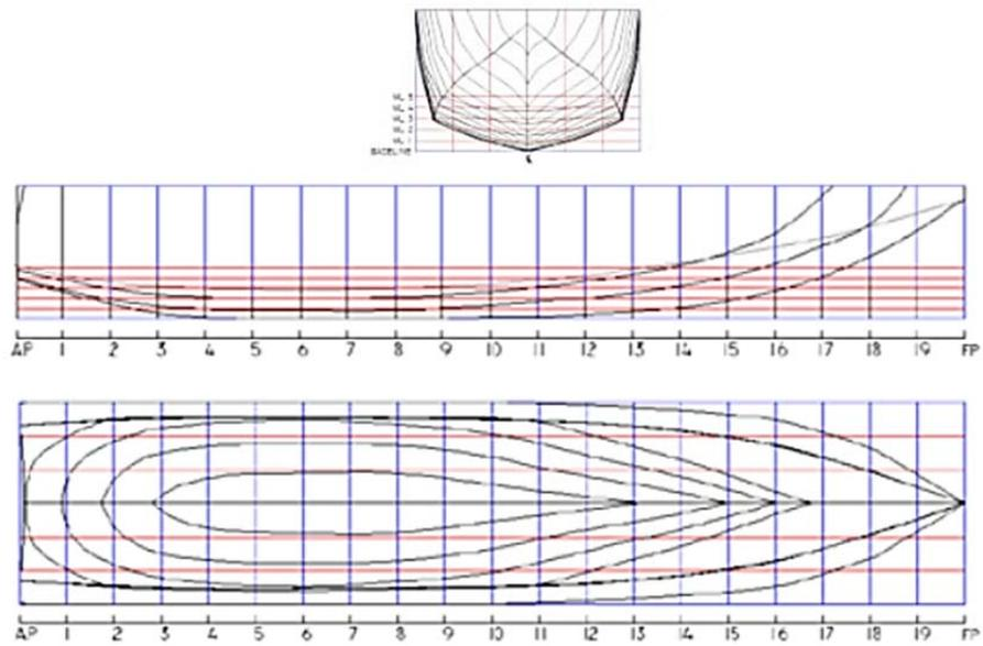
Figure 2 Lines plan of fast patrol boat
