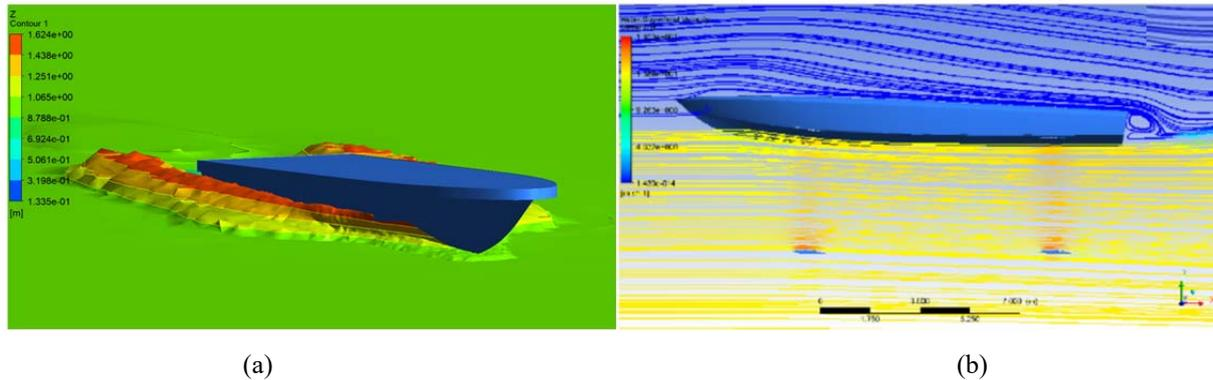
Figure 8 Contour and Streamline visualization of (a) Fast Patrol Boat without Hydrofoil; (a) with Hydrofoil
