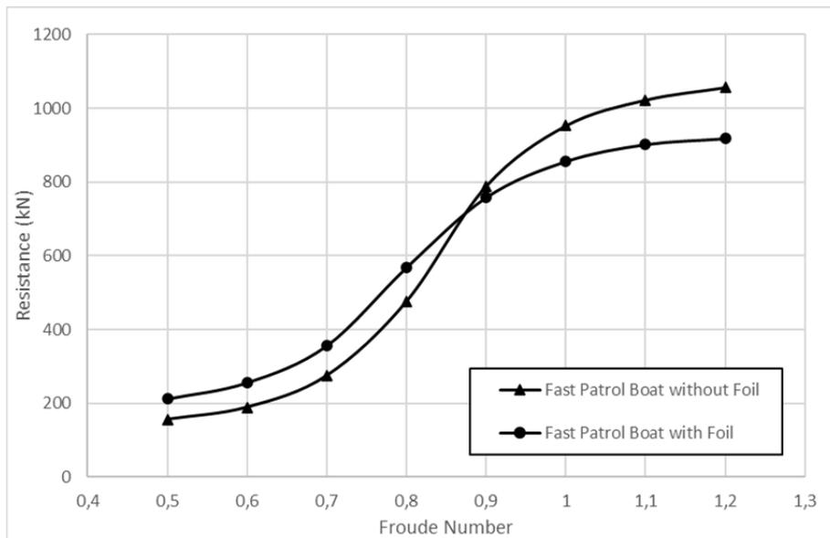
Figure 7 Fast Patrol Boats Resistance using CFD
