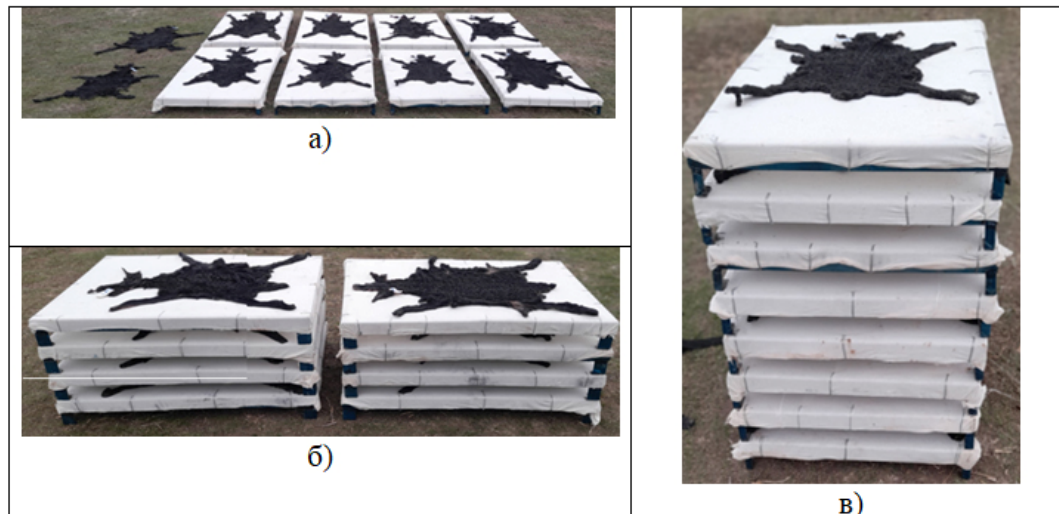
Figure 4. The process of drying karakul without fixing (sticking) to the hygroscopic material of the fixing device: а) the cassettes are laid out; б) cassettes in small groups; в) stack-type cassettes.
