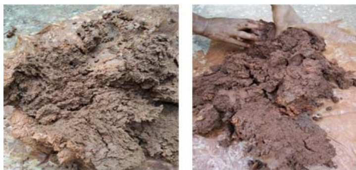
Figure 4 : Paste kneading after fermentation
